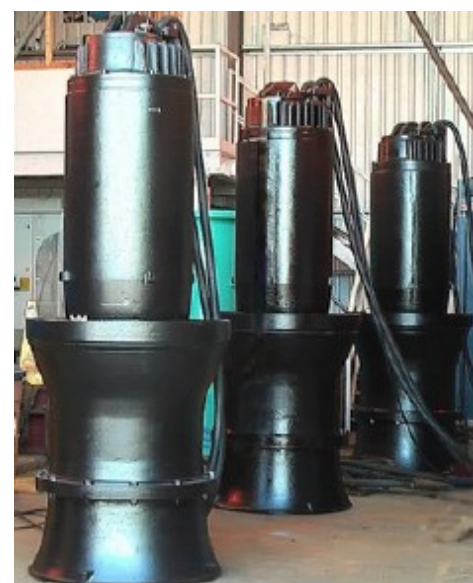
Fig 3. Bedford Pumps replacement pumpsets
